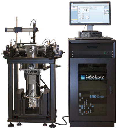
Figure 57 Cryogenic sample holder enables testing samples at temperatures as low as 15 K and under a vacuum.
